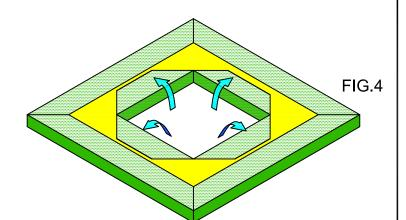
FIG.4: FOLD THE FABRIC TO THE BACK SIDE AND ADHERE IT TO THE FIBERGLASS WITH A SUITABLE SPRAY ADHESIVE.
