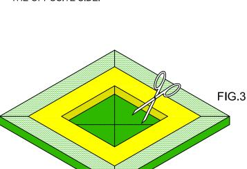
FIG.3: ONCE THE FABRIC IS REVEALED, CUT AN "X" IN THE FABRIC, FROM INSIDE CORNER TO INSIDE CORNER.
