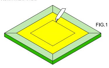
FIG.1: MEASURE THE LOCATION OF THE CUT-OUT AND MARK THE BACK OF THE PANEL. DOUBLE CHECK YOUR WORK. REMEMBER THAT WHEN MARKING THE BACK OF THE PANEL, THE CUT OUT IS ON THE OPPOSITE SIDE.
