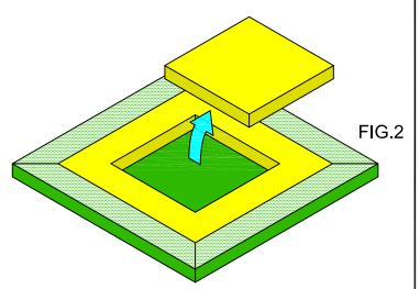
FIG.2: CUT THE FIBERGLASS WITH A RAZOR KNIFE, BEING CAREFUL TO KEEP THE BLADE VERTICAL. DO NOT CUT THE FABRIC AT THIS TIME. YOU CAN CUT THE FIBERGLASS IN LAYERS AND PEEL IT AWAY AS YOU GET CLOSER TO THE FABRIC.
